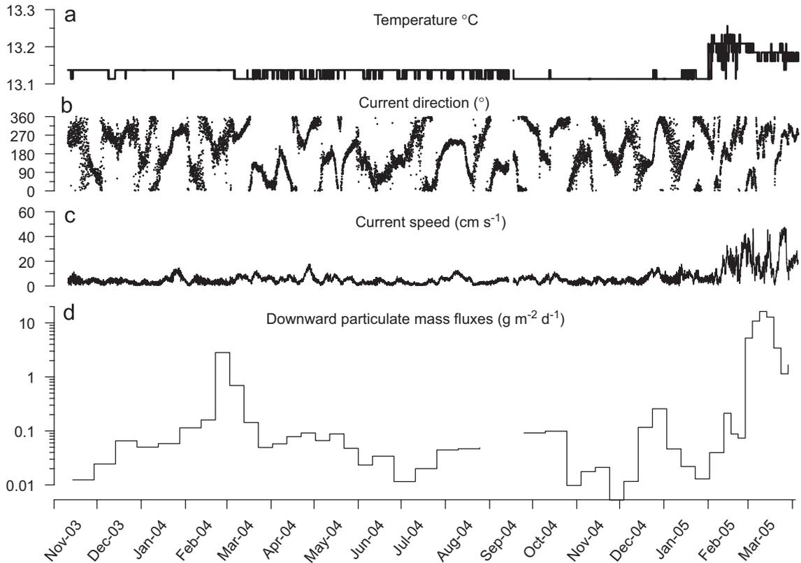
**Fig. 2.** Time series of (a) temperature, (b) current direction, and (c) current speed recorded 220 mab and (d) downward particle mass fluxes collected 250 mab at the basin site during the study period. See location in Fig. 1.
