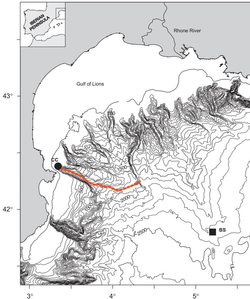
**Fig. 1.** Bathymetry map of the Gulf of Lions showing the location of the basin site (BS) mooring (square) and the Cap de Creus (CC) canyon head mooring site (circle). The axis of the CC submarine canyon is represented by a discontinuous line.
