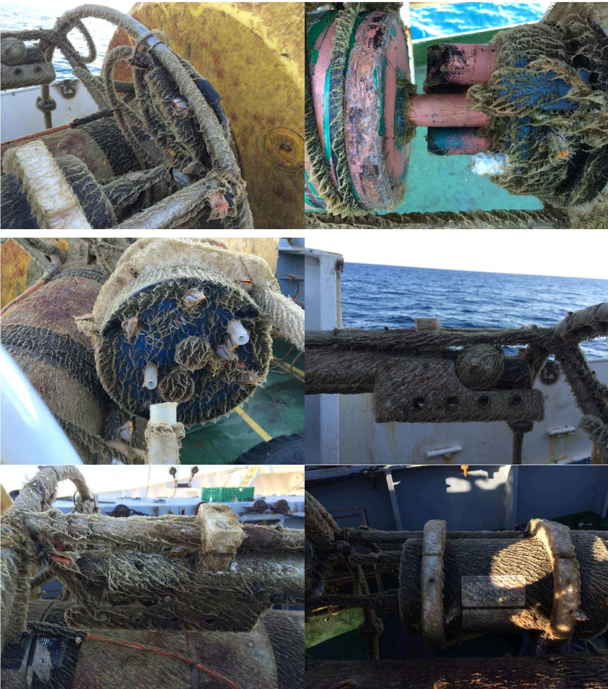
**Figure 7.3.2 a)** Instruments check after recovering, notice the high biofouling on them
