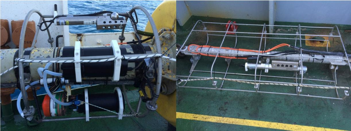
*Figure 7.3.2 b) Cleaned instruments ready to be re-deployed*
