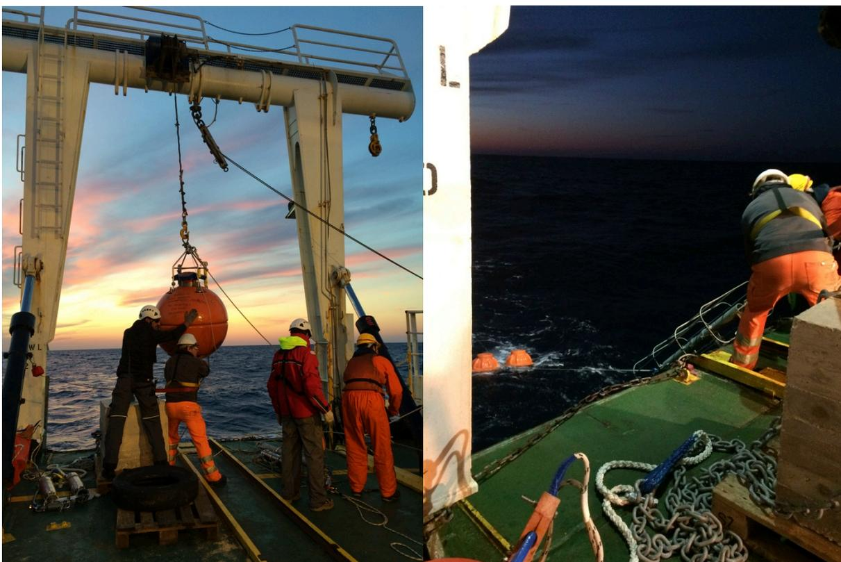
**Figure 7.1.1** Recovering of ADCP with flotation buoy and cage
