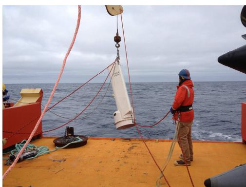
**Figure X** (above). SARL Technicap time-series sediment trap “Frenchie” deployed from LM GOULD, 31 Jan. 2013.
