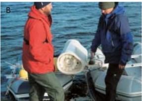
Fig. 5. **A**: A Technicap sediment trap on the ice at Lake E prior to deployment; 26 April 2001. **B**: A sediment trap lying on the improvised raft prior to redeployment in August 2001; the collecting bottles are clearly visible.
